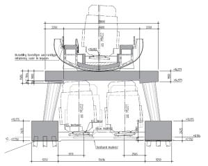
Fig. 1 Table pier over two tracks
