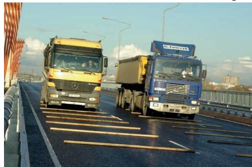
*Figure 1.1 Dynamic load testing done by passing trucks*
