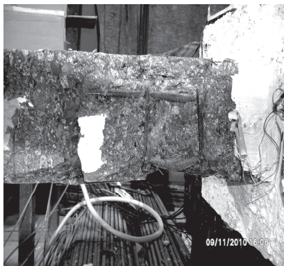
Fig. 1: Specimen S2-3C when displacement is 120 mm
